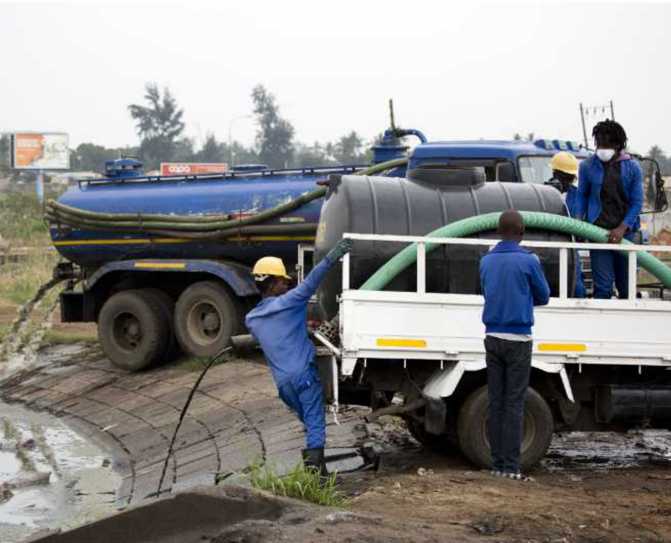
Workers from the community-based organization ACADEC contracted by Water and Sanitation for the Urban Poor (WSUP) discard sewage from a tank on their truck into the Infulene waste water treatment plant in Maputo, Mozambique.
